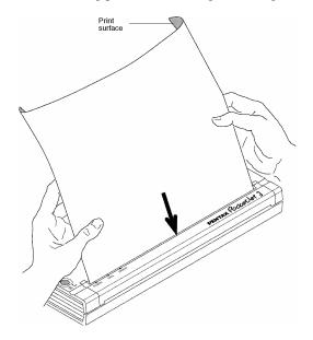
FIGURE 14. Inserting paper
